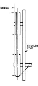
FIXED SHEAVE Fig. 36 — Sheave Alignment
